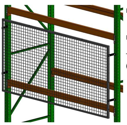
Material Required – Rack Guard Panel and Offset/Flush Mount Clips
